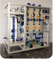
The key point of the EDM technology is to have good monovalent selective membranes to allow the proper separation of monovalent ions from the divalent ones, which are the most susceptible to form insoluble salts. Fuji-
