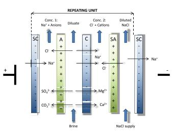
Thanks to this new EDM configuration, the sparingly soluble salts such as CaSO4, MgSO4 or CaCO3, are not produced in neither of the concentrate streams.
